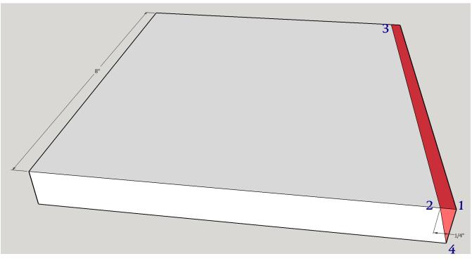
From point 1, measure 1/4" down to point 2. Draw a line from point 2 to point 3. Draw a line from point 2 to point 4. Cut along this angled line the length of the 8" board. Red part is not used.
