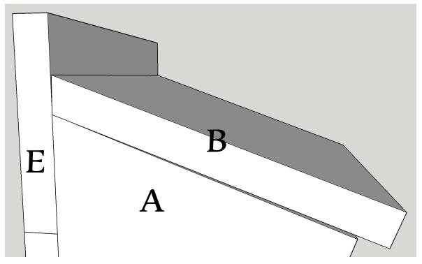
Align the Roof (Part B) with the Back #2 (Part E) and Sides (Part A).
