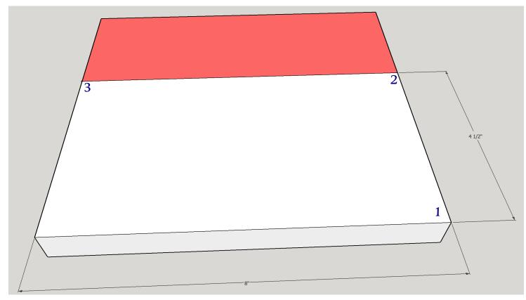
From point 1, measure 4-1/2" down to point 2. Draw a line from point 2 to point 3. Cut along this line. Red part is not used.
